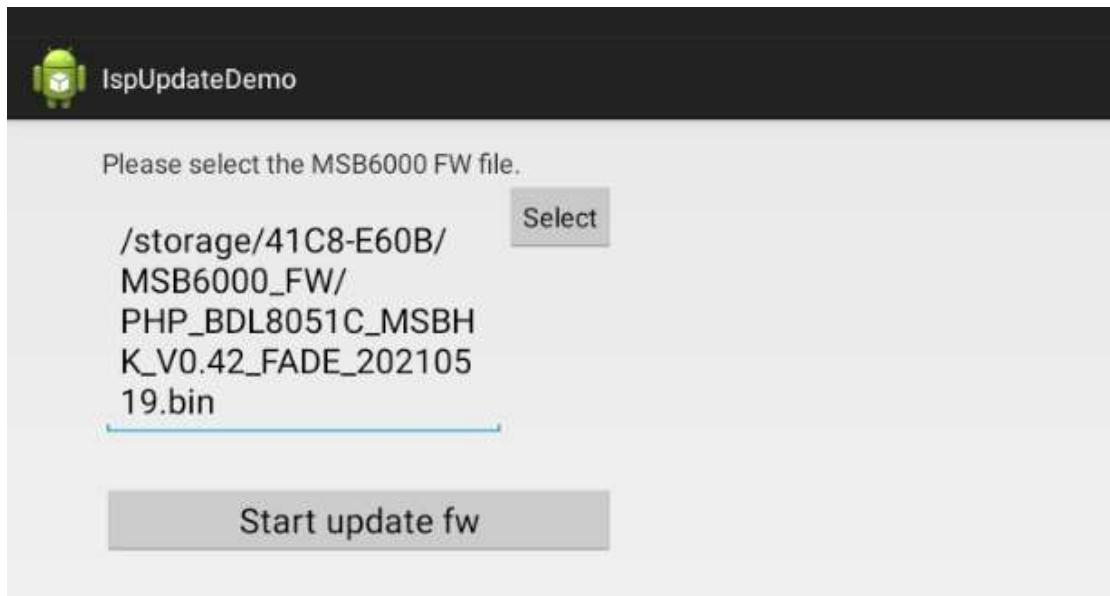
Step5: Press “Start update fw” button. The system will reboot automatically after the firmware update.
